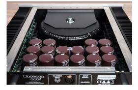
ing capacity up to 160,000 uF for each mono amplifier.
