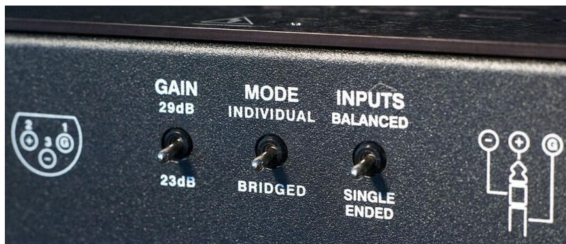
On the back of the Bryston 3B 3 there are toggle switches for selecting the amplification factor, mono-bridged or stereo operation as well as the input selection
