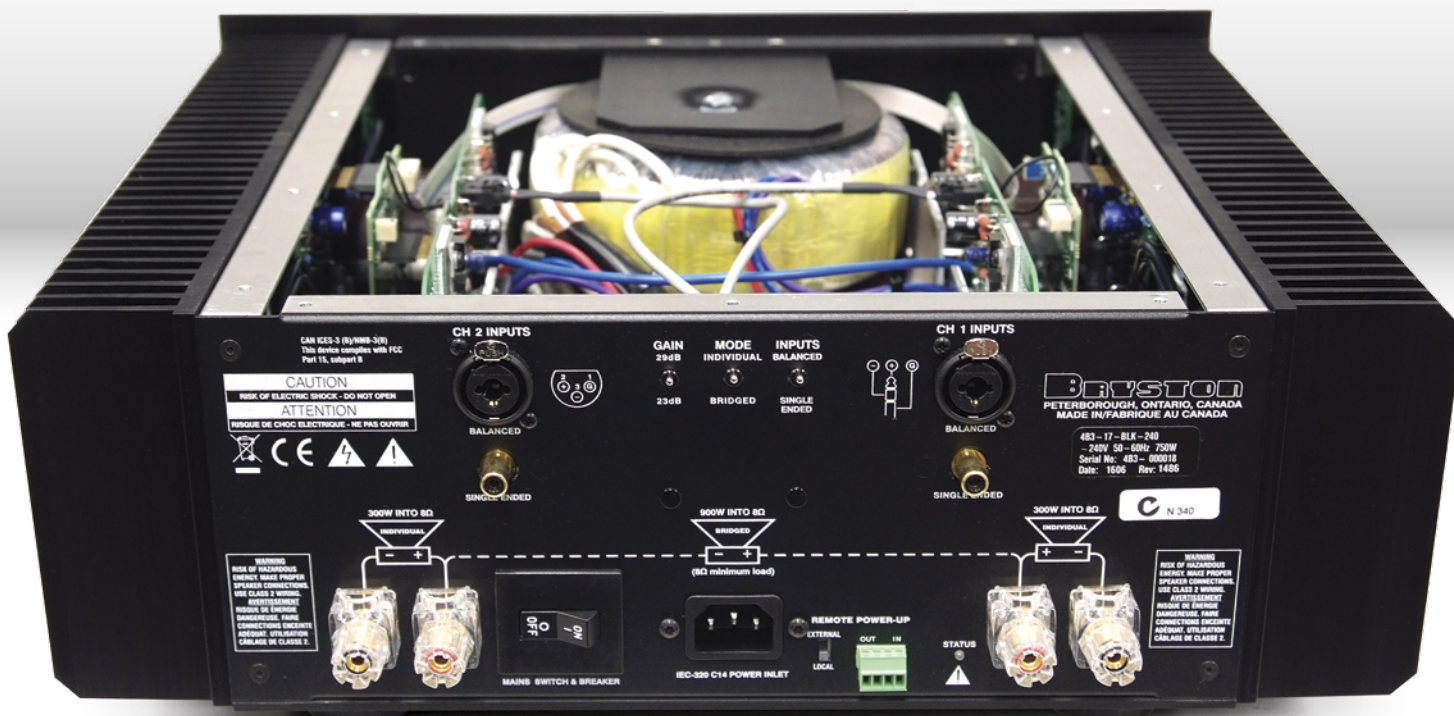
▽ THE SMALL CENTRAL SWITCH TOGGLES THE 4B 3 BETWEEN NORMAL OPERATION AND BRIDGED MONO.
