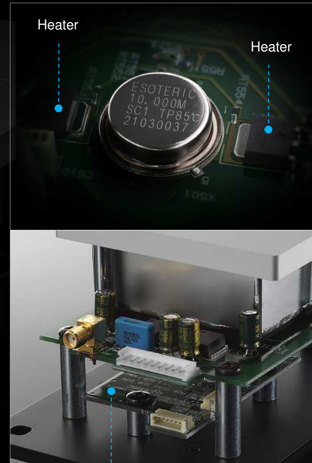
Master Sound TC Control Board That controls heaters
