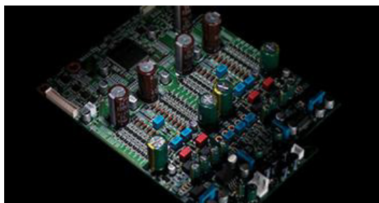
∟ One channel of the MASTER SOUND DISCRETE converter
